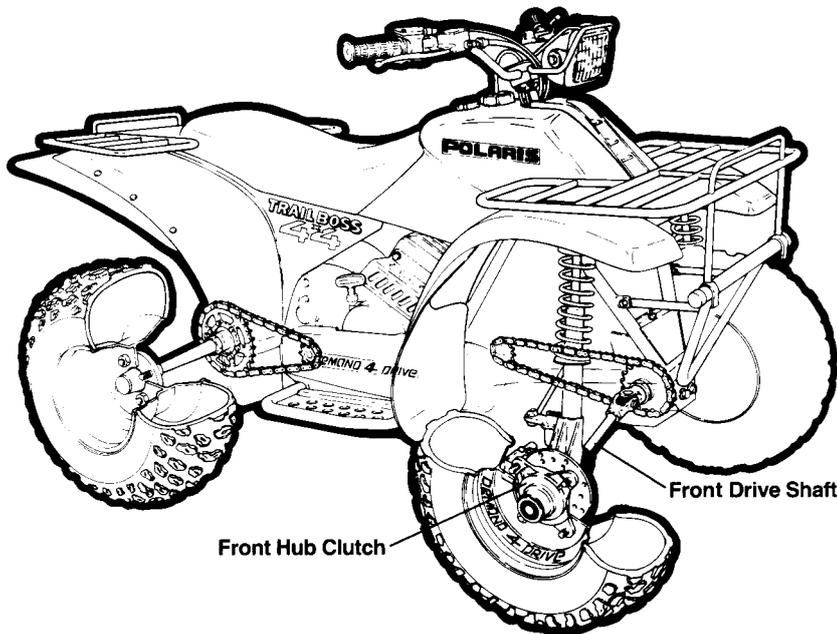
**Front Hub Clutch - Engaged Position**
